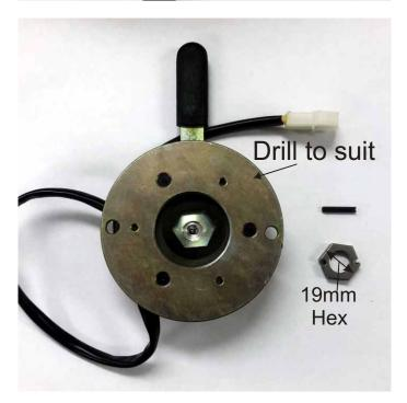
The hex nut is 19mm with a 12mm bore and 3mm roll pin. It may be possible to use your original brake pad and hex in this brake if the thickness is +/- 5mm
